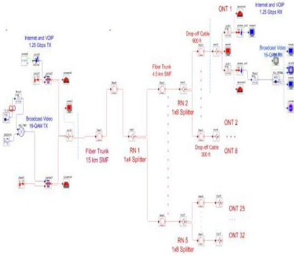
Figure2. Schematic of FTTH-BPON system
