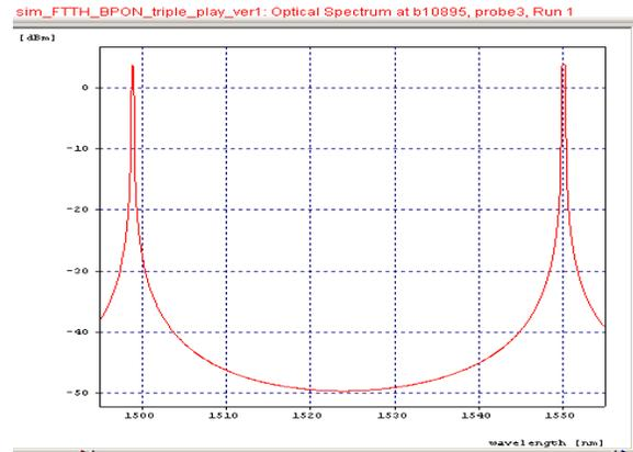
Figure3. Output spectrum from Central Office
