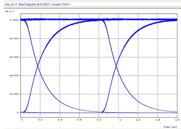
Figure4. Received eye diagram for voice and data signal
