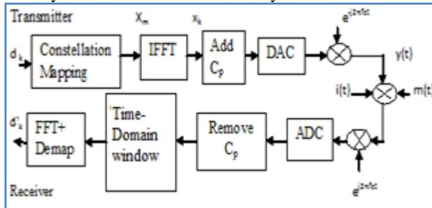
Figure 1. OFDM transceiver.
