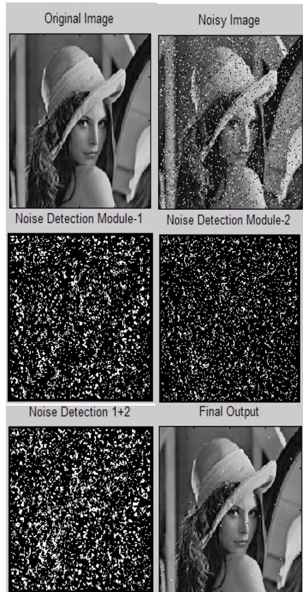
Fig. 4 Process of Restoration of noisy Lena image (256*256) after 30% of impulse noise (salt and pepper noise).
