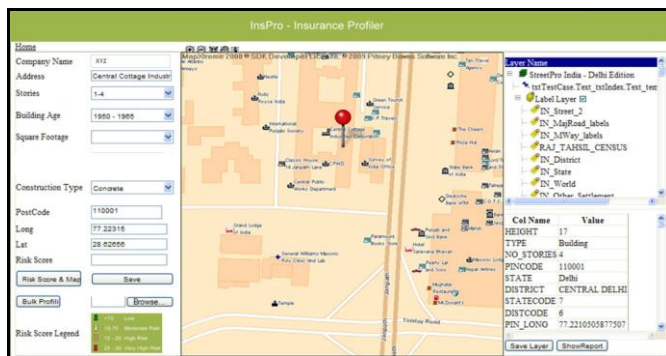
Fig. 4 Insurance Profiler (InsPro) - Web based mapping solution for Insurers/Re-insurers
