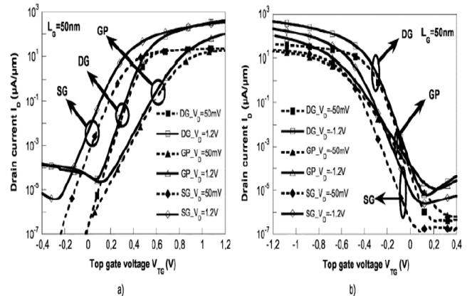
Fig. 1.12 Drain current versus gate voltage for SG, DG, and GP (Ground Plane) transistors with a gate length of 50 nm for both (a) nMOSFETs and (b) pMOSFETs. Source: Julie Widiez et. al.[65]
