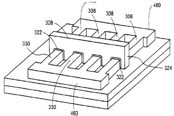
Figure 2(b) completed tri gate MOSFET.
