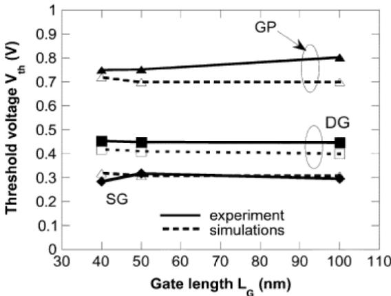
Fig. 1.13 Threshold voltage as a function of the gate length at  $V_{ds} = 50$  mV for nMOS devices. Dashed lines are simulations. Source: Julie Widiez et. al.[65]
