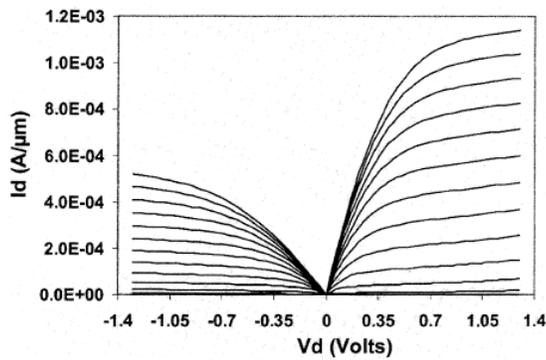
Figure 4. The gate voltage was ramped to 1.3 V in increments of 0.1 V.
