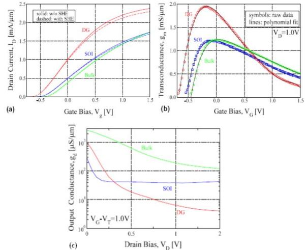
Fig 1.11 (a)  $I_D$ - $V_G$  characteristics (b) Corresponding transconductance curves for the same devices ( $g_m$ ) (c) Drain-bias dependence of  $g_d$  is typically low in saturation but non-zero. Source: Wei Ma and Savas Kaya [64]
