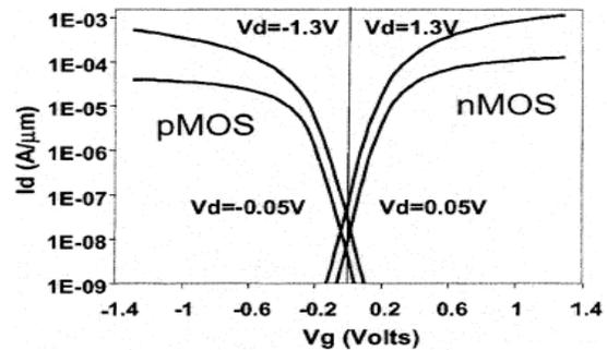
Figure 3. I–V characteristics of 60 nm gate length NMOS and PMOS transistors. The current I is normalized to the width (Z) in all cases.
