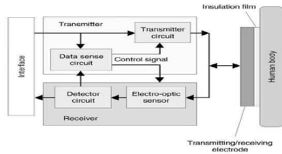
The output of the electro-optic sensor is given to the detector circuit, which in turn given to the interface of the receiving Red Tacton device. The experimental setup for intra body communication assuming communication between two electronic devices (PDAs) is shown in the figure below:
