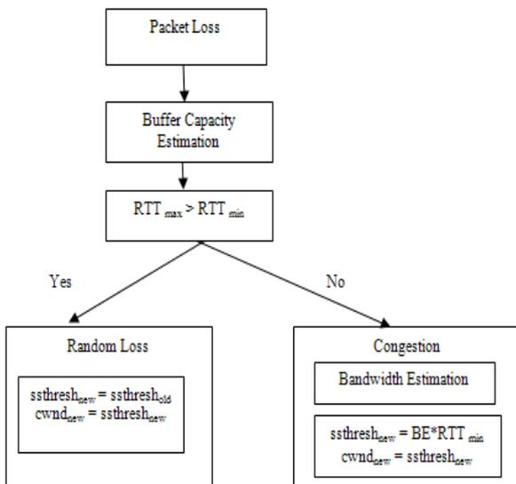
Fig1 : Diagrammatic view of the proposed algorithm
