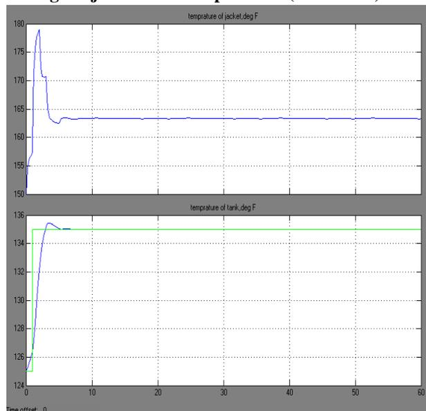
**Figure 9: Output waveform after change in jacket inlet temperature**
