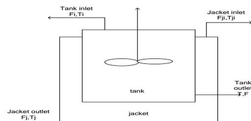
Figure 1: stirred tank heater
