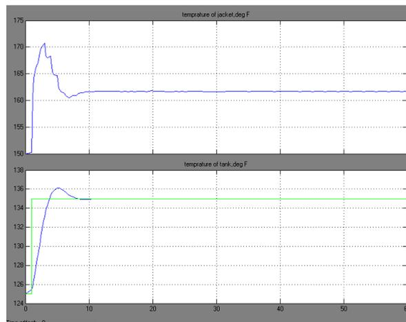
**Figure 8: Output waveform after change in tank inlet temperature**
