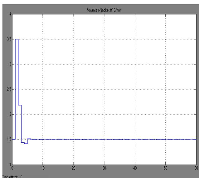
**Figure 11: Manipulated waveform after change in jacket inlet temperature**
