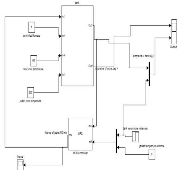
Figure 3: simulation diagram of MPC control
