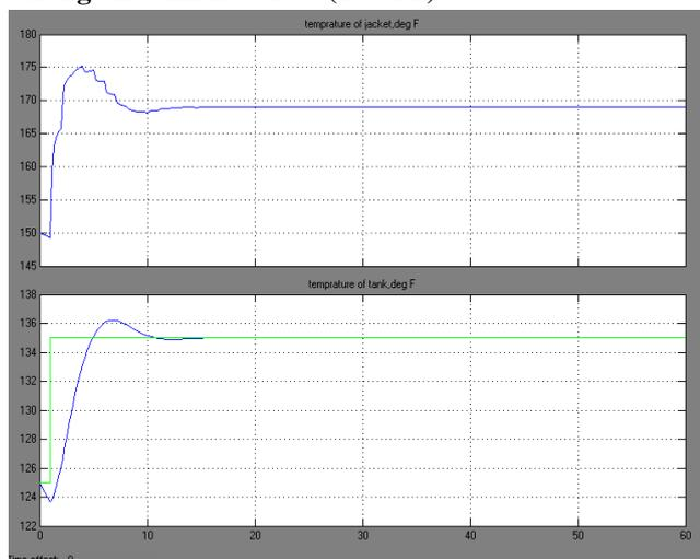
**Figure 6: Output waveform after change in tank inlet flowrate**
