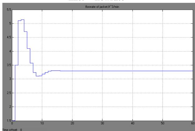
**Figure 7: Manipulated waveform after change in tank inlet flowrate**
