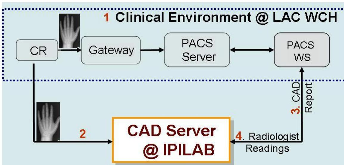
Figure 3. Workflow of CAD implementation at LAC WCH
