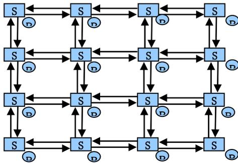
Figure-1 4 x 4 Mesh Architecture
