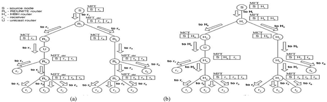
Fig. 2. Data distribution in the Recursive Unicast approach. (a) REUNITE tree. (b) HBH tree.
