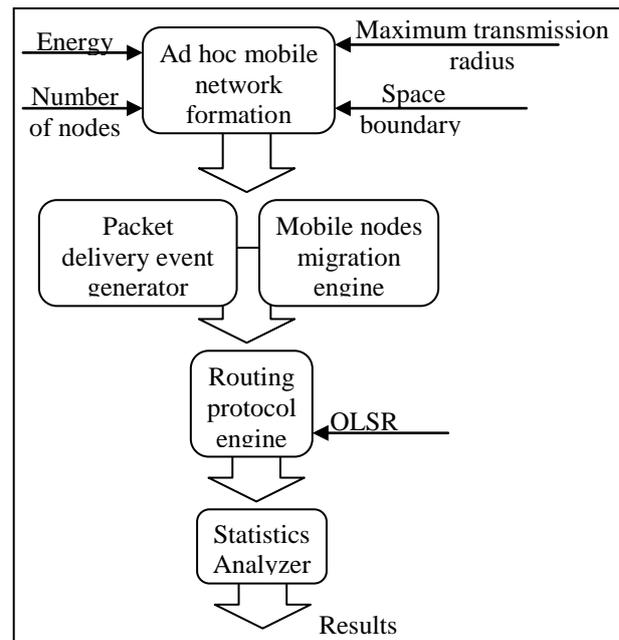
Fig. 1 An ad hoc mobile network simulation model.
