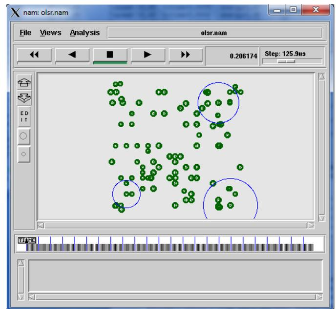
Fig. 2 A sample topology generated by ns-2 Hundred Node Case
