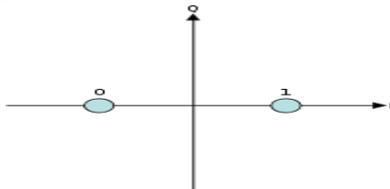
Fig1 Constellation diagram example for BPSK
