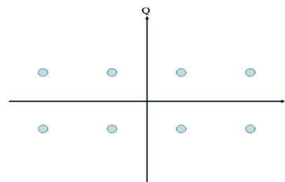
Fig 3 Constellation diagram of 8-QAM system
