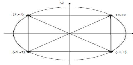
Fig 2: Constellation diagram of a QPSK system
