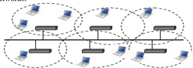
**Fig-1 (Wireless Network Structures-I (Infrastructure Networks))**
