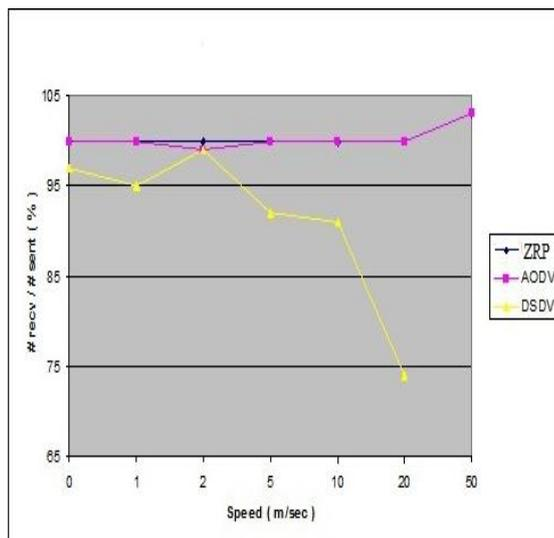
**Fig-4 (Throughput vs Speed)**
