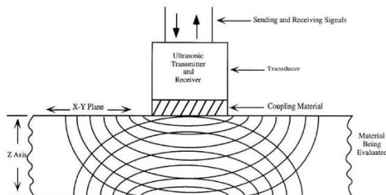
Fig 3: Ultrasonic Transceiver Scanning System
