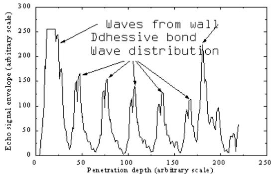
Fig 8: Wave distribution obtained during simulation
