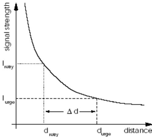
Figure: Signal Levels for Handover
