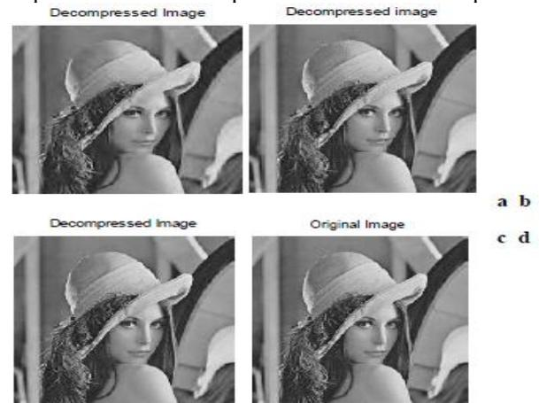
**Fig 2: (a) Original Image of size 512x512 before compression, (b) Decompressed Image using NLIC, (c) Decompressed Image using SPIHT with DWT (d) Decompressed Image using RLE with DCT**
