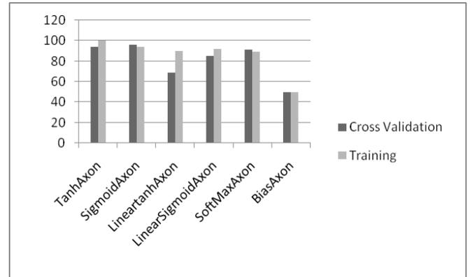
Fig. 2. Variation of % average classification accuracy with Transfer Function for MLP
