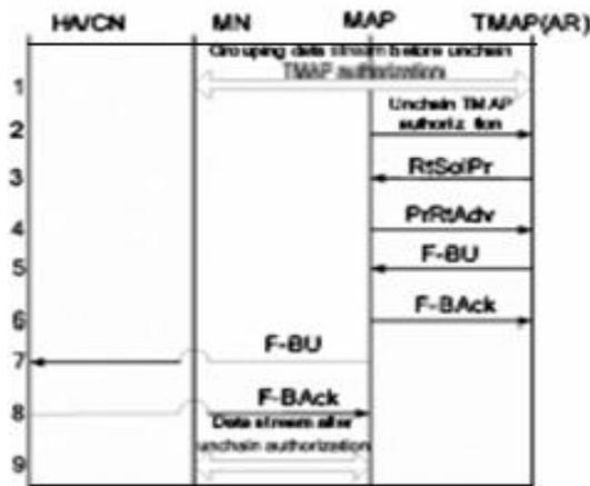
Fig. 3 TMAP unchain authorization process
