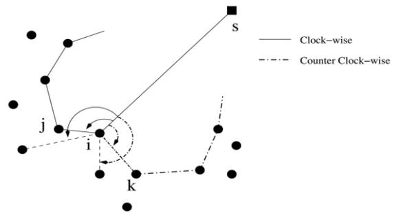
Fig. 2. Illustration of angle-based routing.
