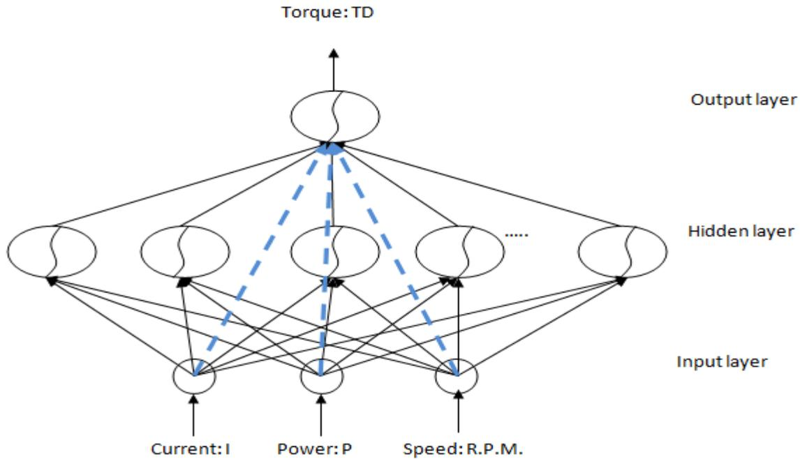
Fig. 2: shows cascade feed forward artificial neural networks: a three layer network has connections from layer 1 to layer 2, layer 2 to layer 3, and layer 1 to layer 3. The three layer network also has connections from the input to all three layers.
