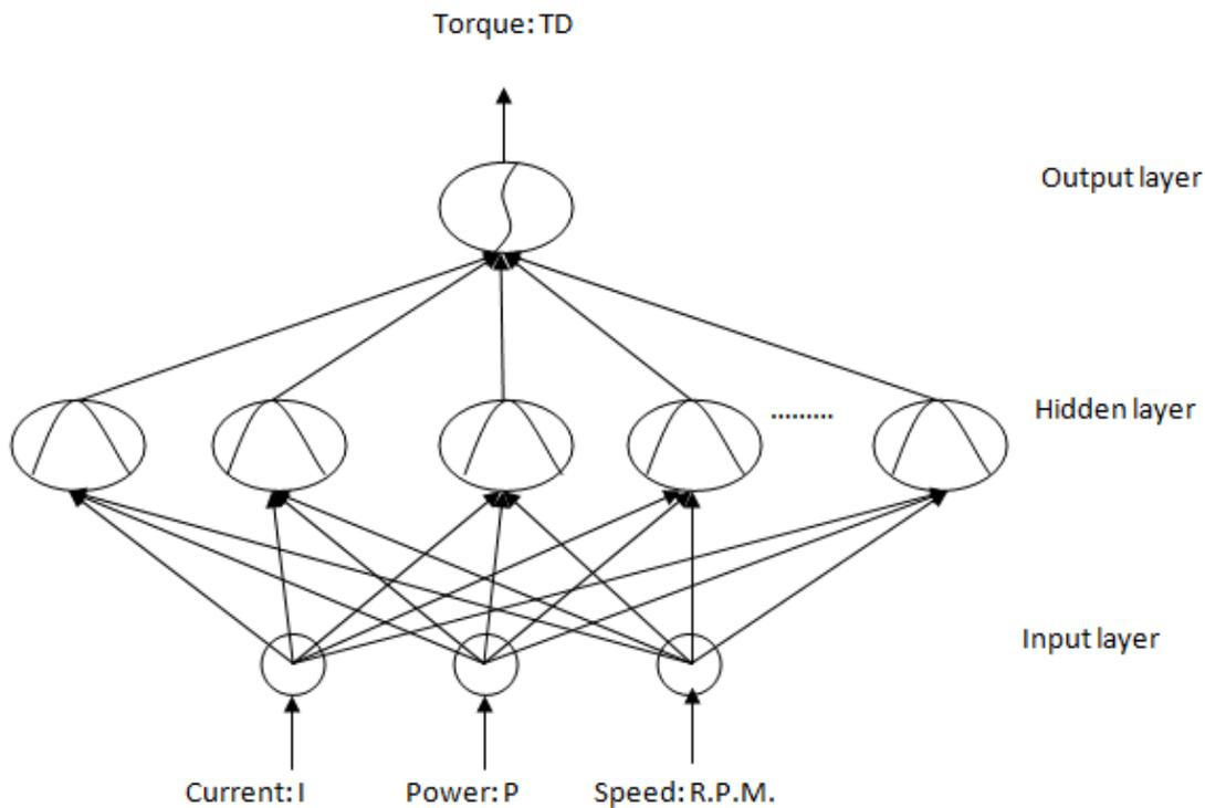
Fig 3: shows radial basis function neural network with the Gaussian function in the hidden layer neurons.
