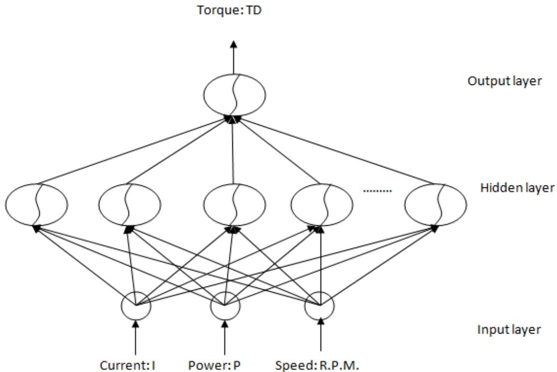
Fig 1: the above network allows signals to travel one way only; from the input to the hidden layer and then to the output layer. There is no feedback i.e. the output of any layer does not affect that same layer.
