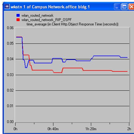
Figure 9: Client HTTP Object Response Time (Sec)
