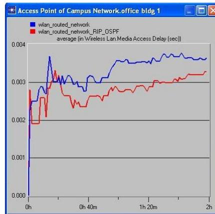
Figure 6: Wireless LAN Media Access delay (Sec)
