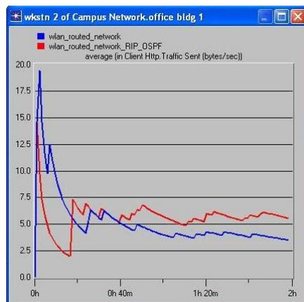
Figure 10: Client HTTP Traffic Sent (bytes/sec)
