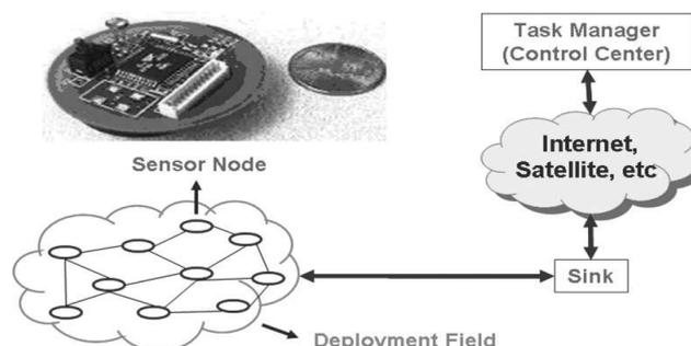
Fig. 1. An illustrated architecture of wireless sensor networks
