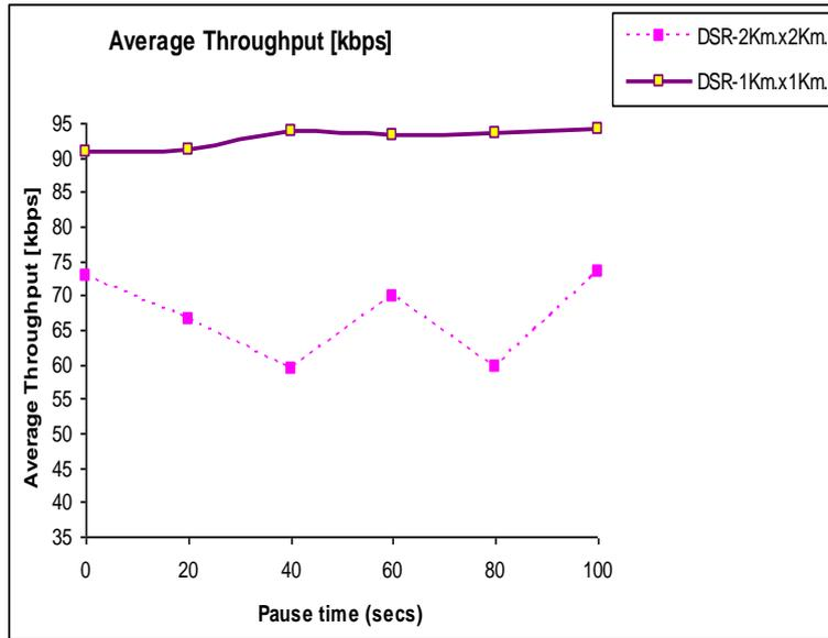
Fig 4: Pause time versus Average Throughput (kbps) when terrain areas are 1 Km. x 1 Km., 2 Km. x 2 Km for DSR.
