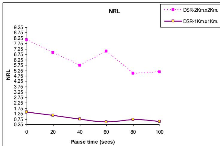
Fig 5: Pause time versus normalized routing load(NRL).when terrain areas are 1 Km. x 1 Km., 2 Km. x 2 Km for DSR.
