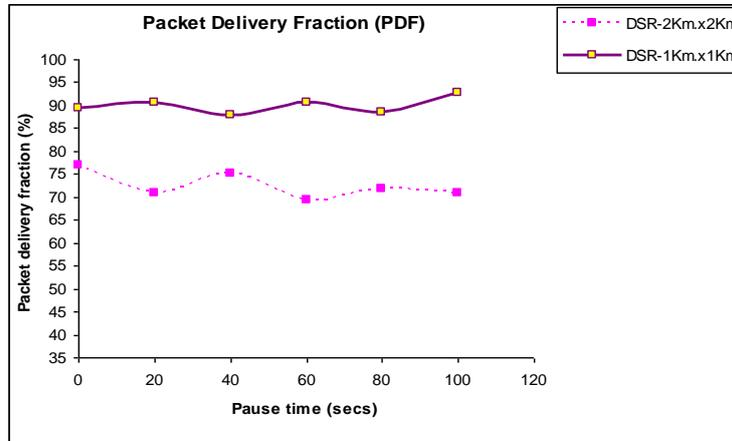
Fig 2: Pause time versus packet delivery fraction when terrain areas are 1 Km. x 1 Km., 2 Km. x 2 Km. for DSR.
