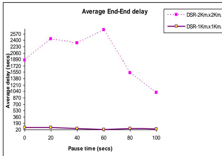
Fig 3: Pause time versus Average End-End Delay when terrain areas is 1 Km. x 1 Km., 2 Km. x 2 Km. for DSR.
