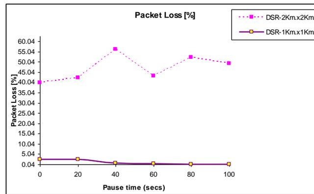
Fig 6: Pause time versus packet loss[%] when terrain areas are 1 Km. x 1 Km., 2 Km. x 2 Km for DSR.
