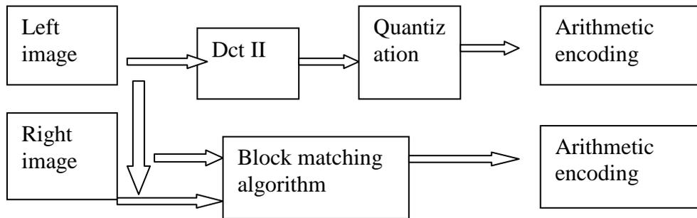
Fig 2. Block based stereo Image encoding process
