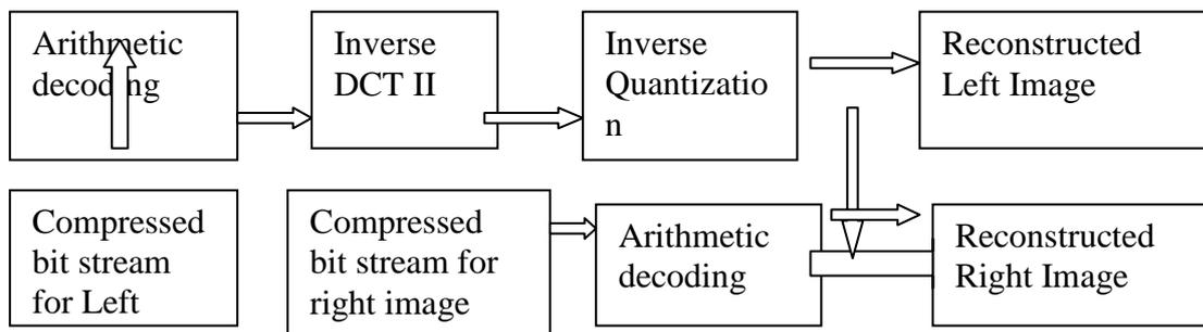
Fig 3. Block based stereo image Decoding process
