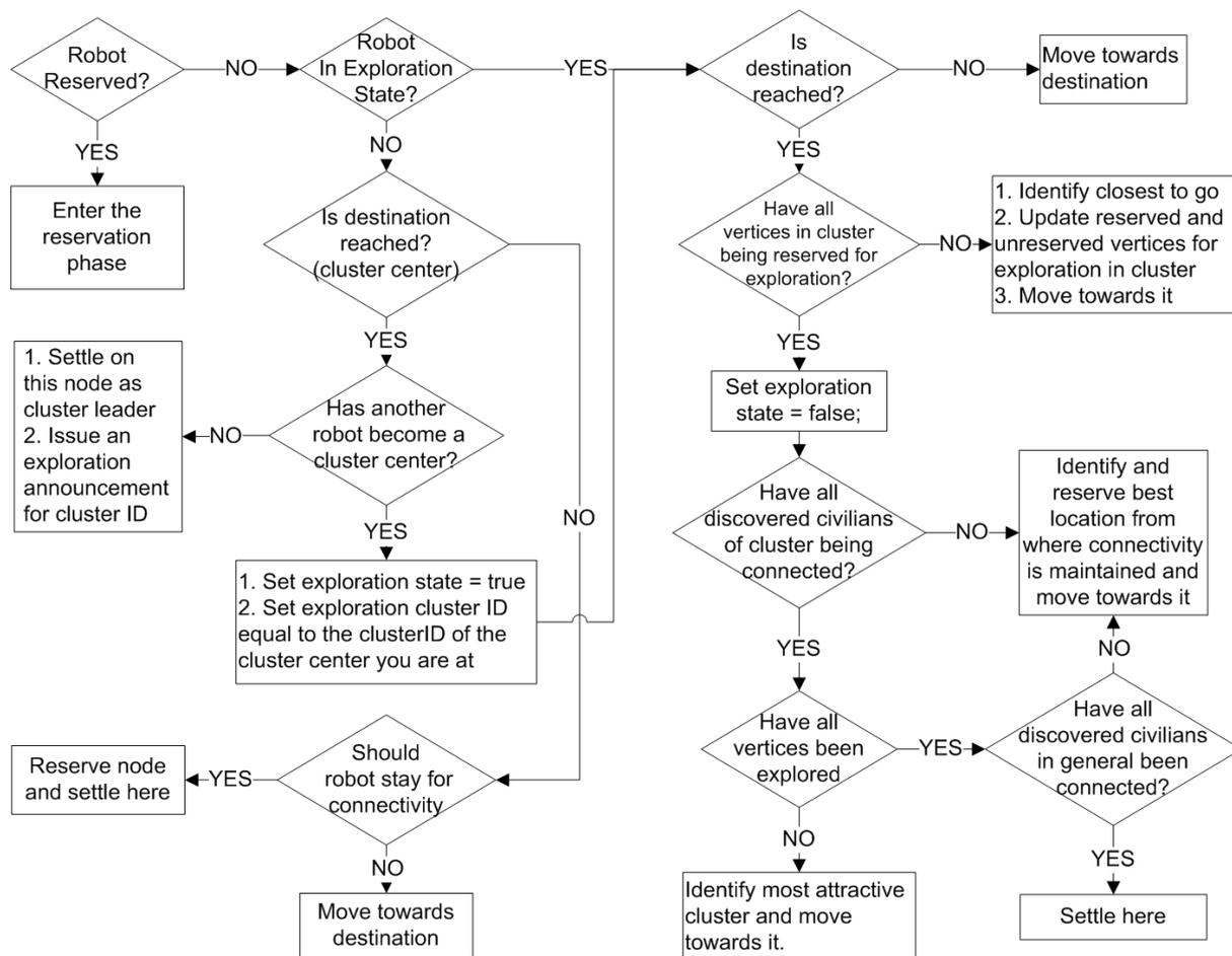
Fig. 3 General flow diagram of the distributed heuristic algorithm
