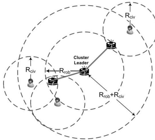
Fig. 4 Connectivity is guaranteed within a cluster if its radius is smaller than  $R_{rob} + R_{civ}$
