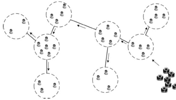
Fig. 6 Illustration of the minimum spanning tree formed by the clusters and the movement options of the robots
