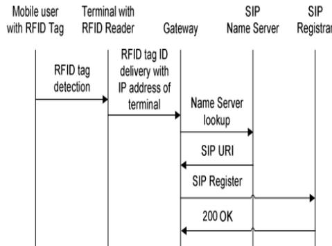
Fig 2: PM registration procedure using RFID[14]
