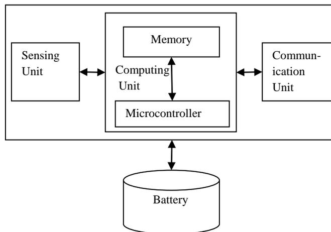
Fig.1 Components of a sensor node
