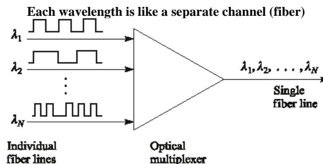
Fig 1.1 Wavelength Division Multiplexing
