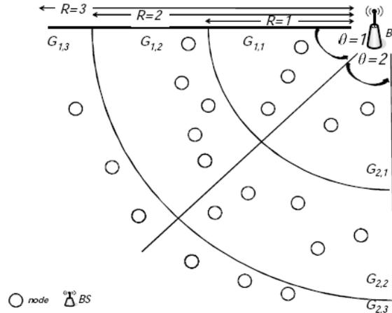
Fig. 2 Grouping example with  $R=1.3$  and  $\theta=1.2$
