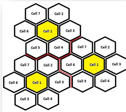
**Fig. 1 Seven-way frequencies reuse cellular system**
