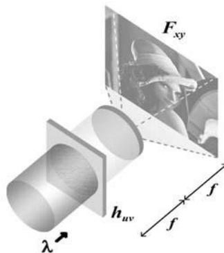
**Figure 4.1** – The relationship between hologram  $h_{uv}$  and image  $F_{xy}$  present at the back focal plane of a lens of focal length  $f$ , when illuminated by coherent monochromatic light of wavelength  $\lambda$ .
