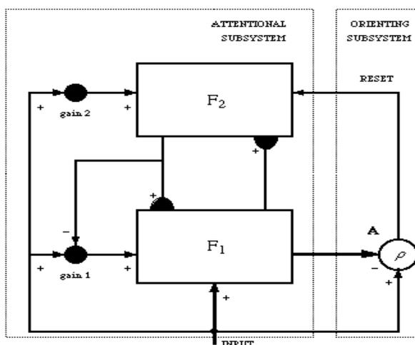
Figure 2. Typical ART neural network block diagram.
