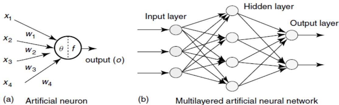
Figure 1: Architecture of an Artificial Neuron and a Multilayered Neural Network
