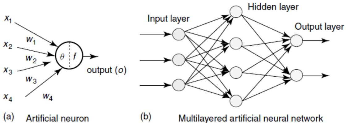
Figure 3: Architecture of an Artificial Neuron and a Multilayered Neural Network
