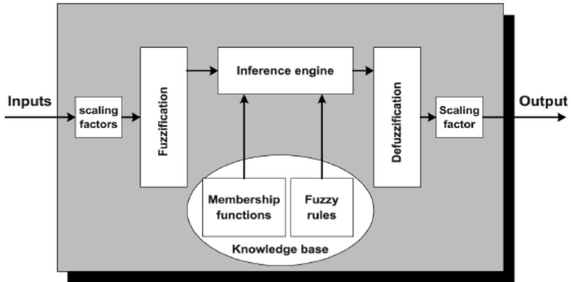
Figure 5: Components of a Fuzzy Logic System
