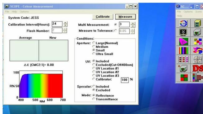
[ Fig.3 COLOR-EYE 7000 E Spectro Measurement Mode]
