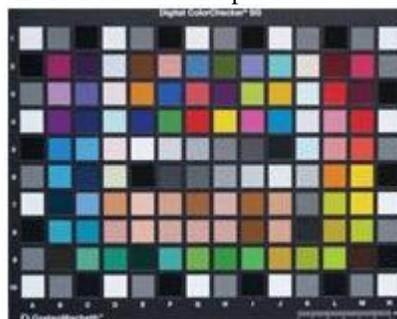
[Fig.4 Color checker X-Rite SGA140 patches]
