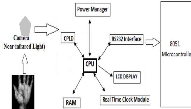
Fig. 4. Architecture of Vein Recognition system
