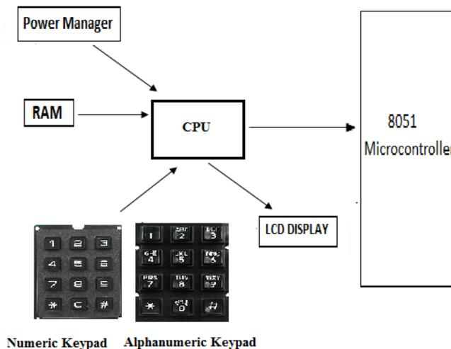
Fig. 5. Architecture of Digital lock
