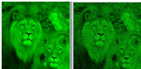
Fig 8: a)Edge Detected using 1-D Prewitt Operator b)Noise Edge Detected using 1-D Prewitt Operator at 50% noise.
