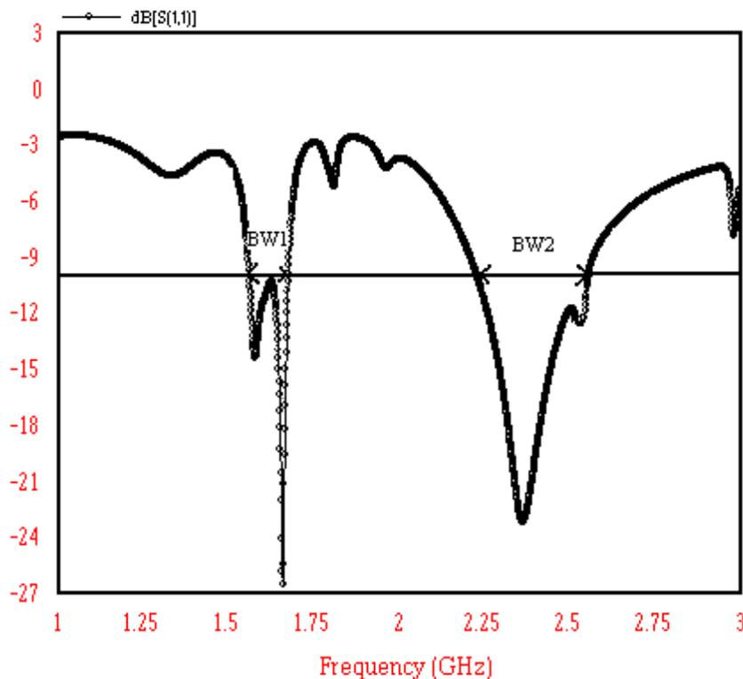
Figure 2. Return loss Vs frequency plot of slotted microstrip antenna.
