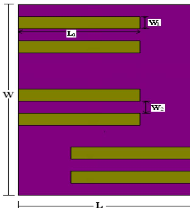
Figure 1. Geometry of proposed microstrip antenna.
