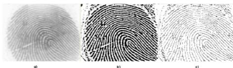
Fig.9 Example of the result of stentiford thinning algorithm applied to a fingerprint image a)fingerprint image b)binarized image c)thin image
