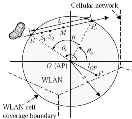
Figure3 Show Travelling Distance Prediction in WLAN cell
