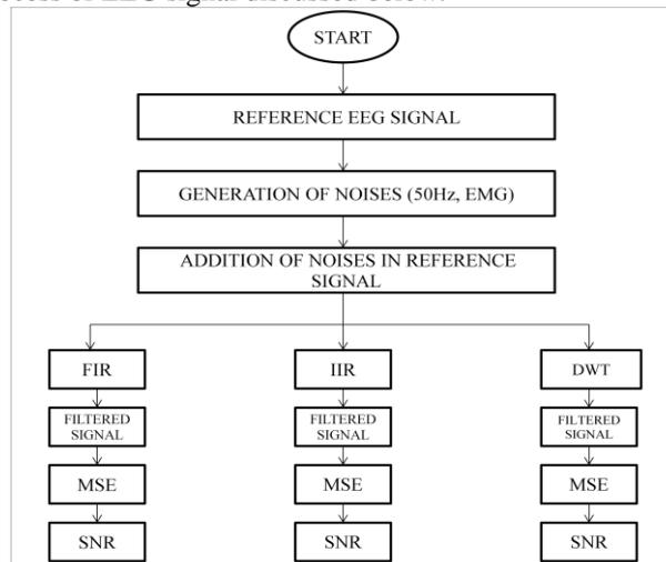
Fig 1 EEG Noising Flow Process
