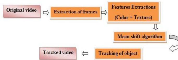
Fig. 1 Main block diagram
