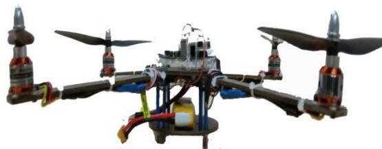
Fig. 3 Side view of Quadcopter
