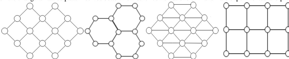
Fig. 2: Rhomboid, Hexagonal, triangular and square grid pattern based node deployment
