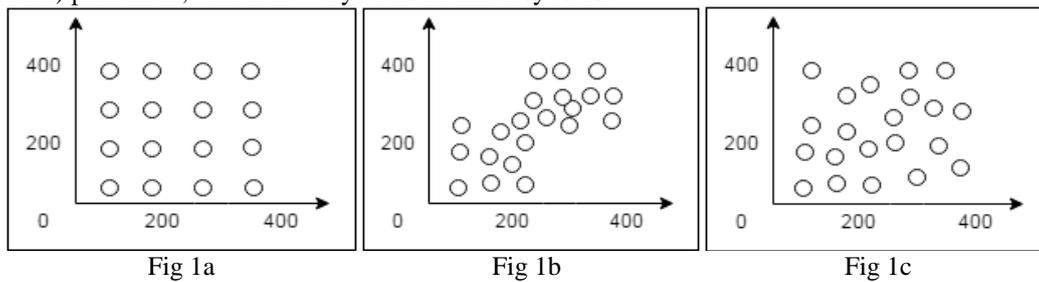
Fig. 1: Grid placement, Biased random placement and non-deterministic placement
