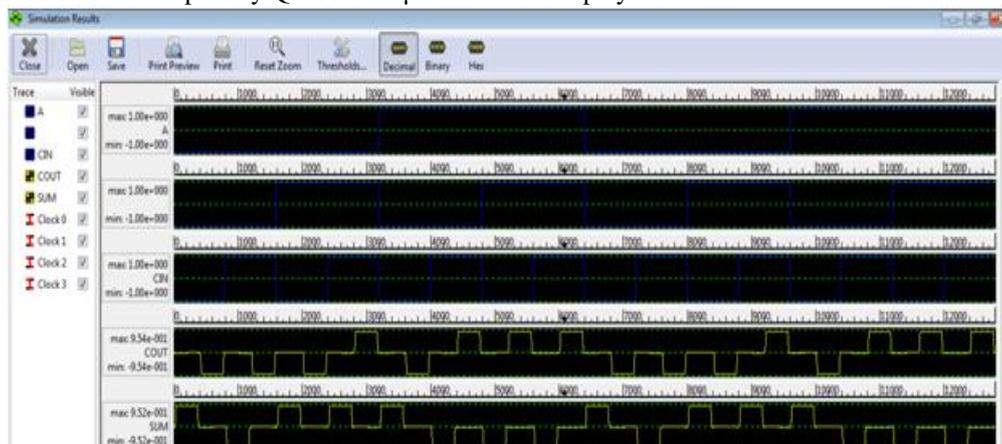
FIG .6 . Input /Output waveform for QFA
