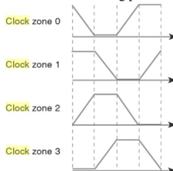
FIG. 4 . Four phases of the QCA Clock
