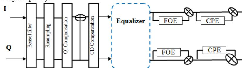
Fig.1 Different Stages of Digital Signal Processing
