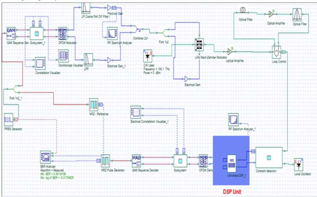
Fig. 1 Implementation of DSP unit for Coherent OFDM System
