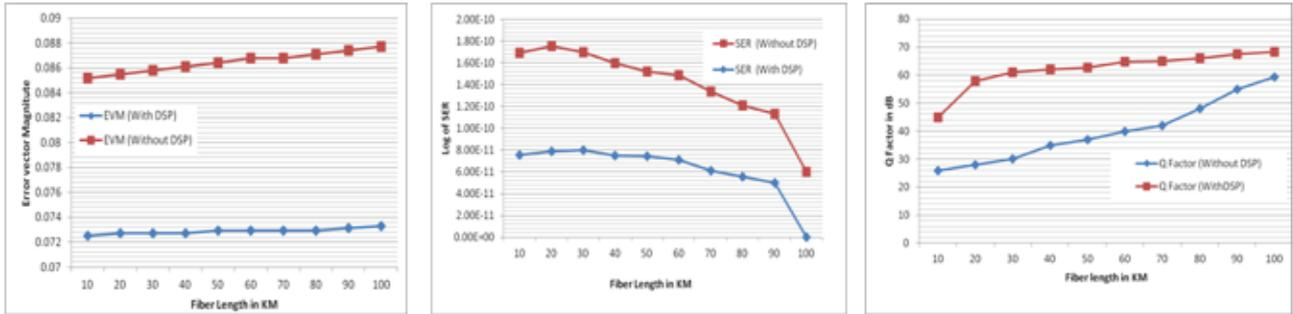
Figure 5.4 Graph for (a) EVM vs Fiber Length (b) SER vs Fiber Length (c) Q factor vs Fiber Length
