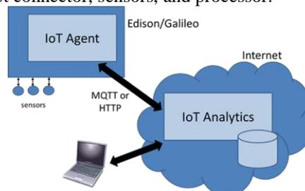
Fig. 3: IOT kit with internet connection and client.
