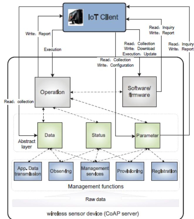
Fig.4: A system architecture of IOT device management including management function, abstract layer and interconnection with client.
