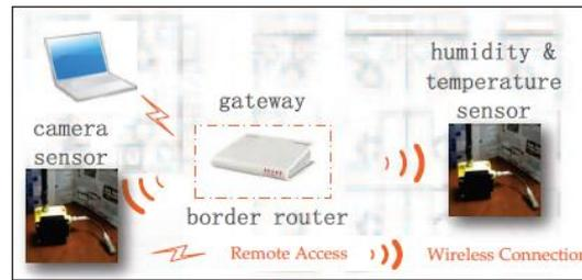
Fig. 2: Network topology of the prototype system. A laptop acts as a client to retrieve sensor resources via gateway.
