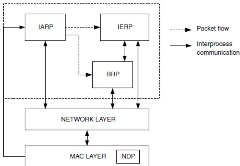
Fig 7: Design diagram of ZRP
