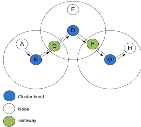
Fig 6: Cluster-head Gateway Switch Routing
